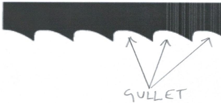
The gullet is there to collect the chips and sawdust and pull it out of the cut. The bigger the gullet the easier it can move the waste out of the cut. So how do you get a bigger gullet? The answer is.....**you need fewer teeth!**
